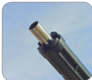
6. Attach a "Drive Socket" to the "Hot Stick" (normally included with standard hot stick kits)
